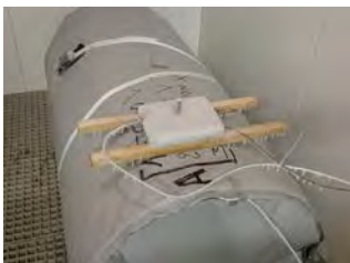
LIFERAFT STORED FOR 50HRS AT -70^{\circ}\text{C}
