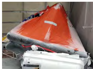
LIFERAFT INFLATED AFTER BEING STORED FOR 50HRS AT -70^{\circ}\text{C}
