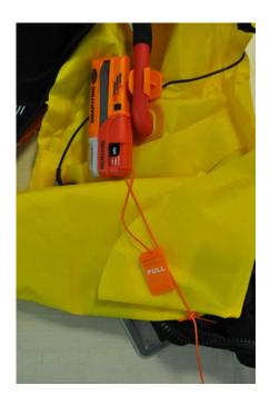
Fold the base of the inflation chamber up towards the S20. Tie the orange lanyard, using 3 half-hitches, around the webbing where the inflation chamber is attached to the cover. Tie off as short as
